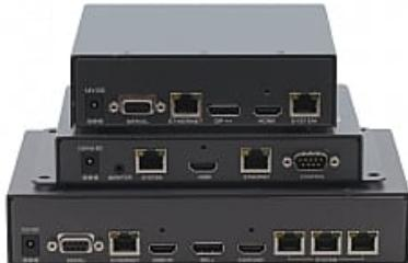
The DS Vision Digital family is an HDBaseT distribution system for HDMI and DisplayPort signals up to 1080p @60, bidirectional RS-232 and Ethernet. The system can distribute the input signals over a single CATx cable from one source to multiple display devices
